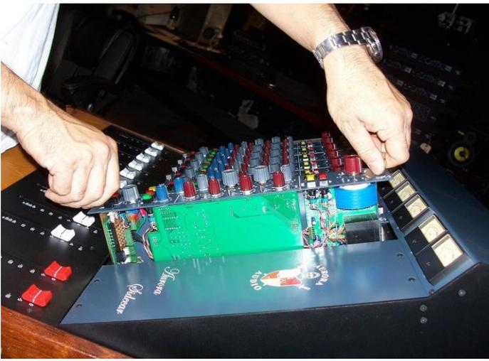
To remove the module, undo the two captive thumb-screws and use them to pull the channel module from its connector and out of the Sidecar frame.
